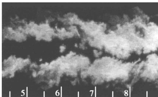
Fig. 7 Second pulse flow image ( t = 100 \mu\text{s} ) showing the structures after pairing.
