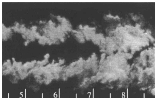
Fig. 9 Second pulse flow image ( t = 100 \mu\text{s} ) showing the merged structures between 7.5D and 9D .
